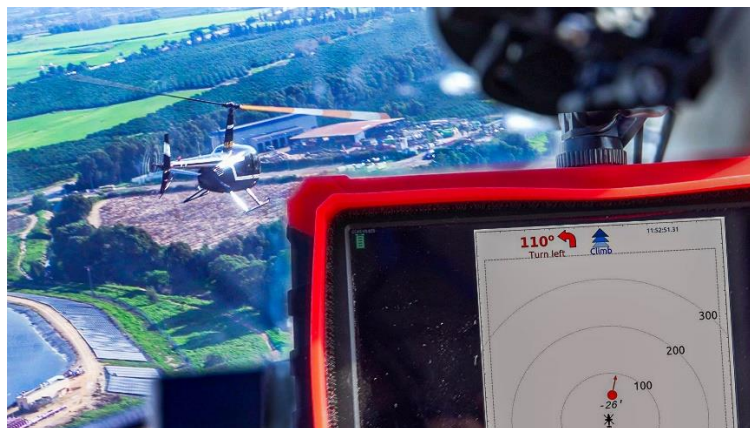
C&CAS flight test onboard 2 helicopters. Dec 2023 Israel. The rare helicopter must turn left and climb to evade a collision.
